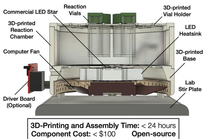
**Figure 1.** Cutaway view of the Wisconsin Photoreactor Platform architecture with labeled components. Estimated component cost is in U.S. dollars as of June 2021.
