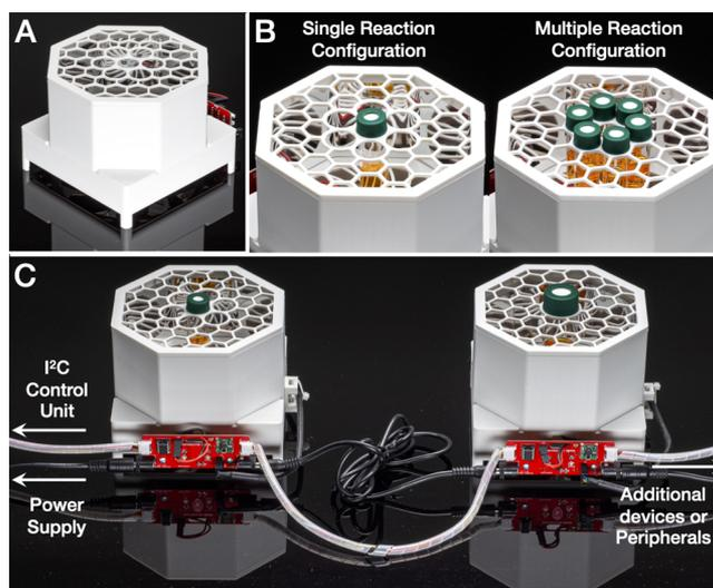
**Figure 3.** (A) Assembled WPP device. (B) Single and multiple reaction configurations of a WPP device fitted with a 4 mL vial holder and reaction chamber module. (C) Illustration of WPP expandability using optional driver boards.
