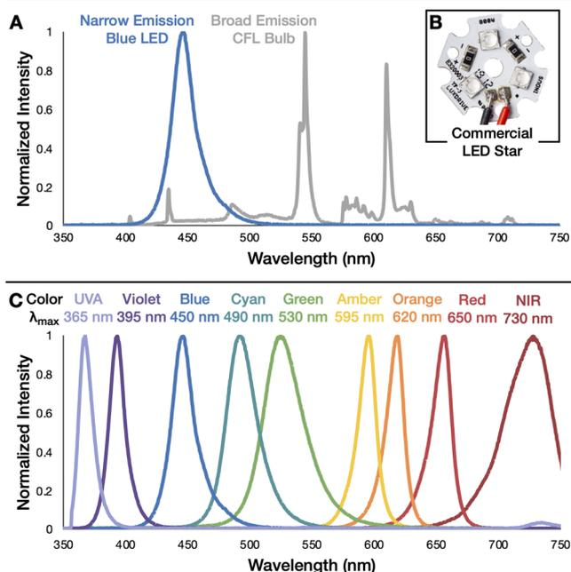
**Figure 2.** (A) Comparison of emission spectra of 450 nm Cree, Inc. XT-E royal blue LED and ALZO Digital full spectrum CFL bulb. (B) Industry-standard LED star mounted with 450 nm Cree, Inc. XT-E LEDs. (C) Emission spectra of commercial LEDs purchased from manufacturers Cree, Inc., Luxeon, and Inolux.
