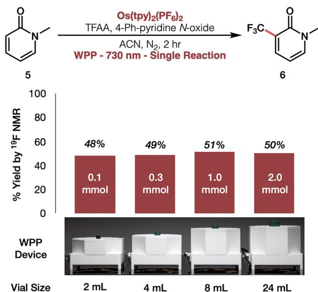
**Figure 5.** Results of scale-up trials. Reactions conducted at indicated scales using listed reaction vessel sizes over 2 hours. Yields were determined by <sup>19</sup>F NMR analysis of crude reaction mixtures using trifluorotoluene as an internal standard.
